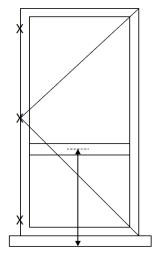
These doors are made to be glazed or have a panel fitted (either full or half panel)
