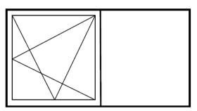
The sash opens in two different ways tilting inwards (hinged from the bottom) which is known as "Tilt" and from the side again opening inward known as "Turn"
