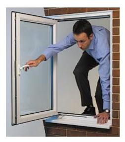
A clear opening of 0.33m2 is required. This must be at least 450mm wide and x 450mm high The bottom of the opening must not be more than 1100mm above the floor
