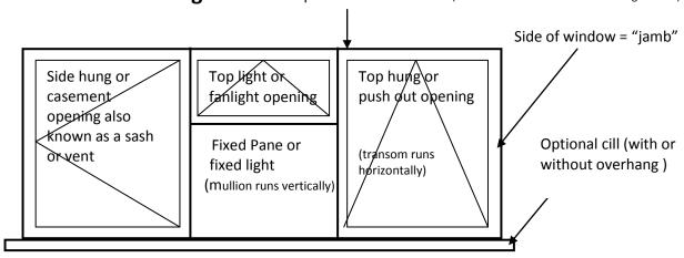
The window drawing shows three different types of opening window
